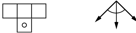
Figure 19. An typical neighborhood for use in a scan with horizontal propagation front, supporting propagation in the direction interval DI[-3\pi/4, -\pi/4] .
