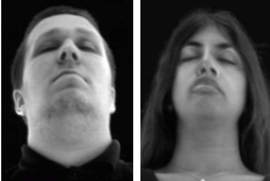
Figure 5.1. Images of summed reflectance map intensities. When the intensities of all samples in a subjects different reflectance maps are summed into corresponding pixel values, and the dynamic range of the result is scaled to a displayable format, this is the result. The female subject's hair was not tied back during measurement in order to test the algorithm. Normally, a measurement where the hair covers the face would be useless.
