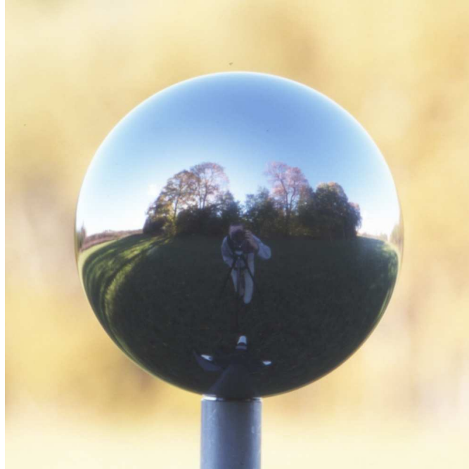
Figure 2.6. The mirroring sphere used to capture illumination environments. The reflection from the area behind the sphere is compressed near the edges of the sphere, and will be captured at a lower resolution than the area in front of the sphere.
