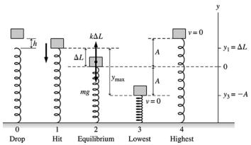
It's essential to carefully visualize the motion. At the highest point of the oscillation the spring is *stretched* upward.
