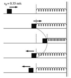
**Solve:** (a) The spring's compression or decompression is one-half of the oscillation cycle. This means the contact time is  $\Delta t = \frac{1}{2}T$ , where *T* is the period. The period is calculated as follows:
