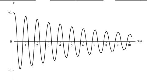
**14.29.** Model: The pendulum is a damped oscillator.
