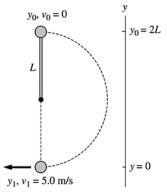
We placed the origin of the coordinate system at the bottom of the arc. **Solve:** We need to find the length of the pendulum. The conservation of mechanical energy equation for the pendulum's fall is  $(K + U_g)_{top} = (K + U_g)_{bottom}$ :
