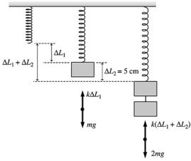
The length of the stretched spring due to a block of mass *m* is  $\Delta L_1$ . In the case of the two block system, the spring is further stretched by an amount  $\Delta L_2$ .
