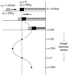
**14.61.** Model: A completely inelastic collision between the two gliders resulting in simple harmonic motion. **Visualize:**
