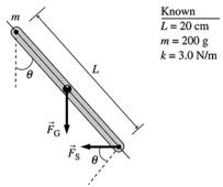
**Solve:** We must derive our own equation for this combination of a pendulum and spring. For small oscillations,  $\vec{F}_s$ remains horizontal. The net torque around the pivot point is
