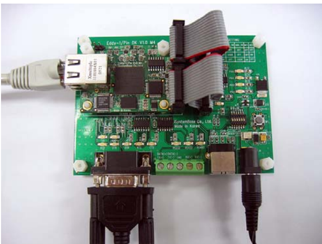
Eddy-S1/Pin attached on the Development Kit Board
