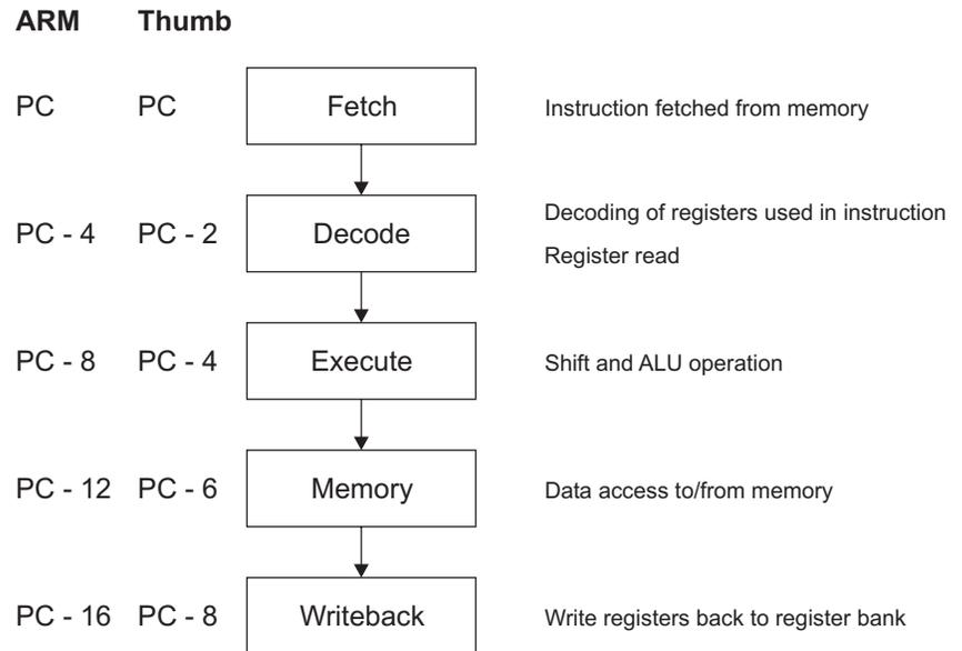
**Figure 1-1 Five-stage pipeline****Note**
