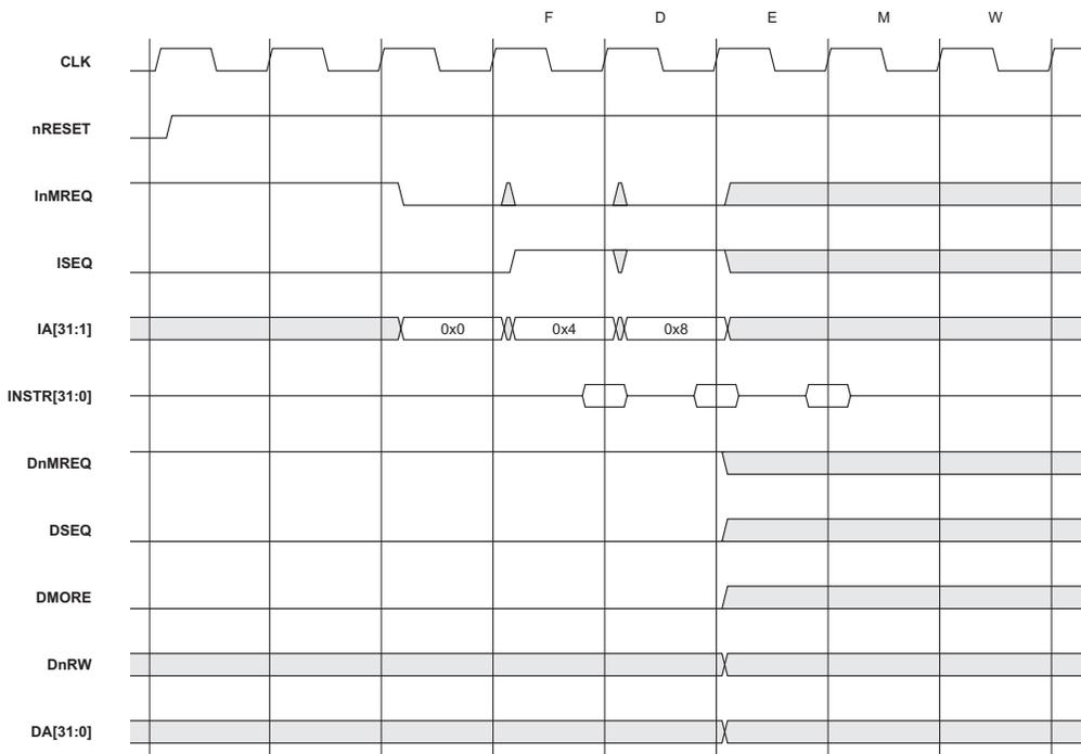
Figure 3-2 ARM9E-S behavior on exit from reset
