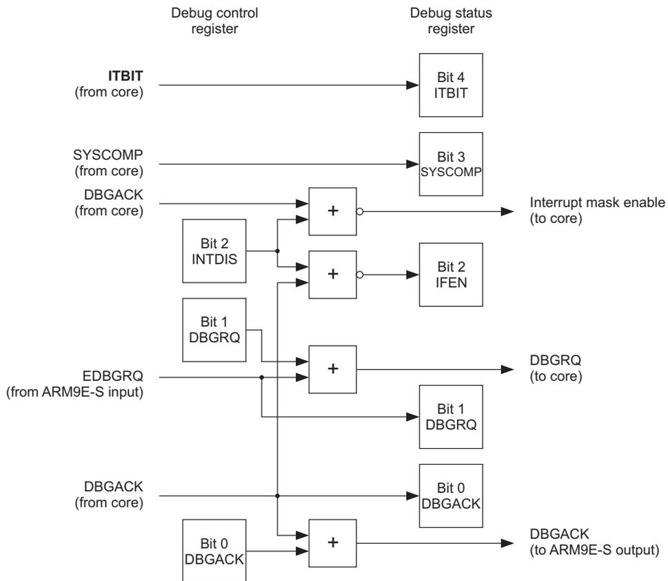
Figure C-12 Debug control and status register structure
