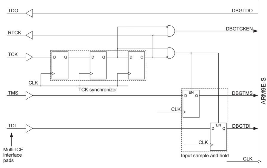
Figure 7-7 Clock synchronization
