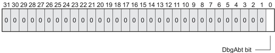
**Figure 7-9 Coprocessor 14 monitor mode debug status register format**
