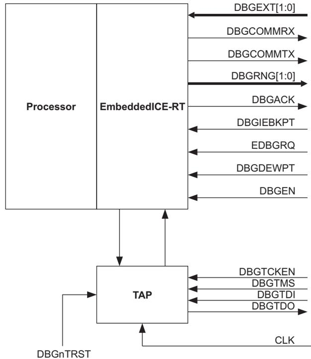
**Figure 7-3 The ARM9E-S, TAP controller, and EmbeddedICE-RT**
