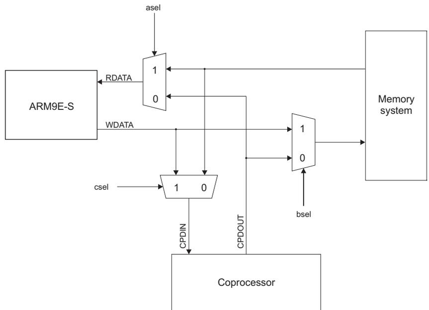
**Figure 6-11 Coprocessor connections**
