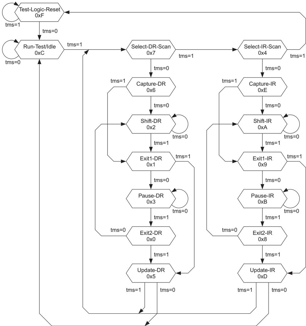
Figure C-2 Test access port controller state transitions<sup>1</sup>
