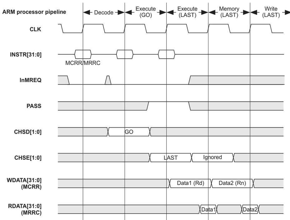
Figure 6-4 ARM9E-S MCRR or MRRC transfer timing
