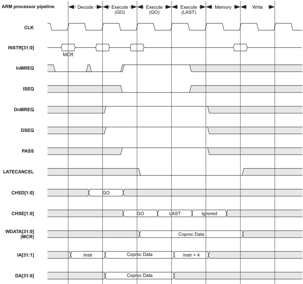
Figure 6-10 ARM9E-S coprocessor 15 MCRs
