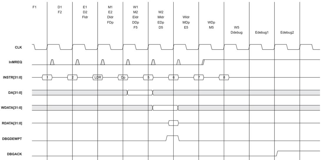
**Figure 7-5 Watchpoint entry with data processing instruction**
